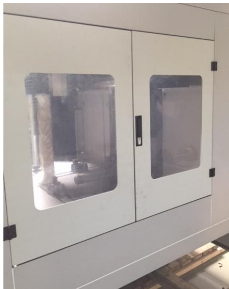
Figure 3.2.16 Side doors must be locked
