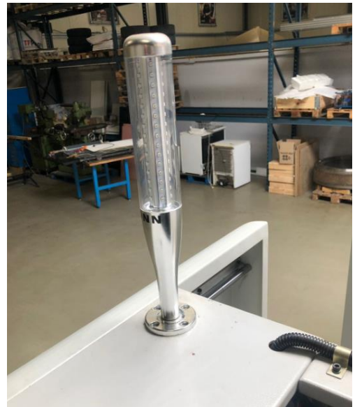
Figure 3.2.8 Mount the lamp
