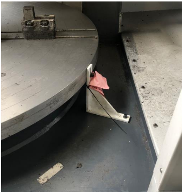
Figure 3.2.13 Dismantle the support
