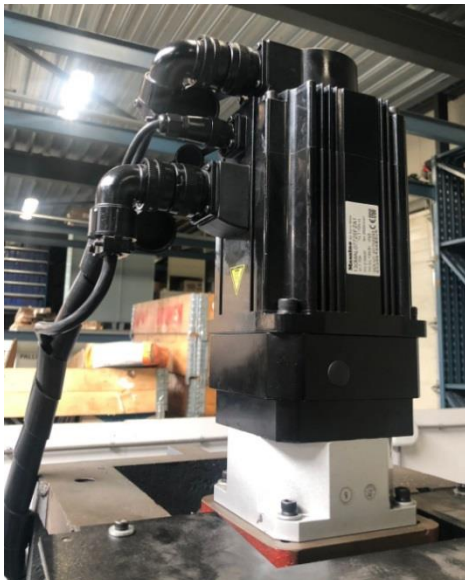
Figure 3.2.9 Mount the servo motor
