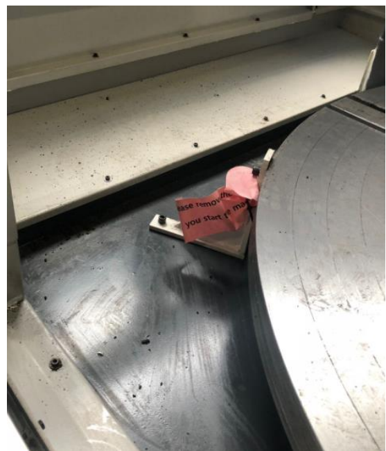
Figure 3.2.14 Dismantle the support
