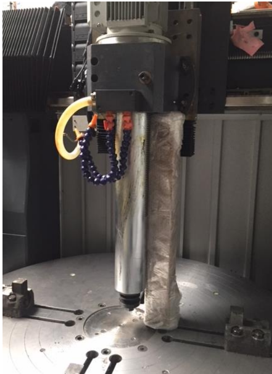
Figure 3.2.15 Remove wooden block
